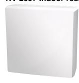
Wall mounted Pt100 sensor for measuring air temperatures indoor. Representative wall box. Precision wire-wound platinum detector. Pt100 sensor connected in a 3 or optional 4 wire system. Single or duplex. Accuracy to IEC 751 class B standard Optional class A, 1/3DIN or 1/10DIN. Temperature range: -10°C to 50°C Optional 4-20mA two-wire transmitter.
