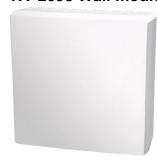
Wall mounted Pt100 sensor for measuring air temperatures indoor. Representative wall box. Precision wire-wound platinum detector. Pt100 sensor connected in a 3 or optional 4 wire system. Single or duplex. Accuracy to IEC 751 class B standard Optional class A, 1/3DIN or 1/10DIN. Temperature range: -10°C to 50°C Including 4-20mA two-wire transmitter.
