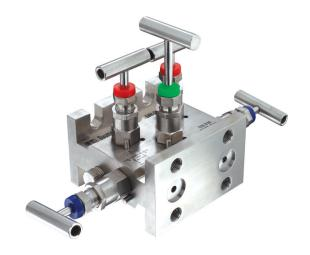
With Flange horizontal port inlets and Flange port outlets. The vent/test ports are positioned on the bottom side. The isolating and venting bonnets are positioned on the left and right hand side and the equalizing bonnet is positioned on the top side. Designed for direct mounting.
