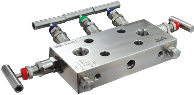
With threaded horizontal port inlets and Flange outlets. Two vent/test connections are positioned on the bottom of the body. The isolating and equalizing bonnets are angular positioned on the top side. The venting bonnets are positioned on the left & right hand side. Designed for direct mounting.
